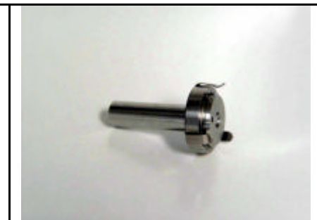
USP/EP App.1 Basket Adapter # 316-3250 depends on instrument (only sets of 6,7,8)
