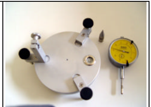
SWT 2 shaft wobble + centricity tester # 30-31210
