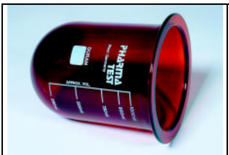
USP amber coloured vessel incl code # 303-5425 (1 litre) # 303-5222 (2 litre) # 302-5622 (4 litre)
